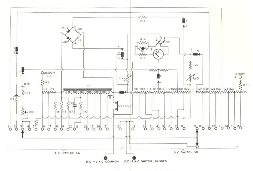
CIRCUIT DIAGRAM OF THE MODEL 8 MK. III AVOMETER
