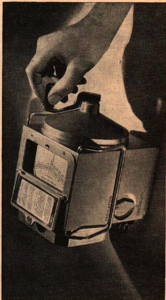
Figure 1. The Meg Insulation and Continuity Tester described on Page 31. Suitable for measuring insulation resistance at 500 volts and conductor resistance at low pressure.
