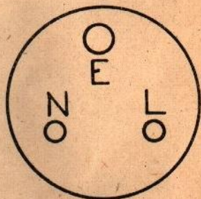
Figure 3. Diagram showing disposition of contacts in a 3-pin socket-outlet as viewed from the front.
