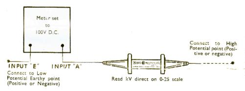
Set the Electronic Multimeter to its 100V D.C. range and connect the short lead of the Multiplier to the INPUT "A" socket of the instrument, Connect the INPUT "E" socket of the instrument to the low potential point of the high voltage source, and connect the long lead of the Multiplier to the high potential point of the voltage source. Set the instrument METER REVERSE Switch for forward deflection of the indicating needle. Full-scale deflection on the Flectronic Multimeter equals 25,000V D.C.
