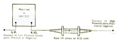
Set the Electronic Test Meter to its 100V D.C. range and connect the short lead of the Multiplier to the X10 socket. Connect the L.P. terminal of the Electronic Test Meter to the low potential point of high voltage source and the long lead of the Multi-plier to the high potential point. Set the METER REVERSE Switch for forward deflection of the indicating needle. Full-scale deflection on the Electronic Test Meter equals 25,000V D.C.
