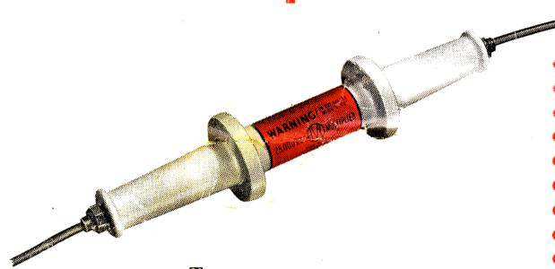
The illustration shows one of the "Avo" 25,000 V D.C. Multipliers which have been designed for use with the Models 8, 8SX, 8X, H.R.1 and H.R.2 AvoMeters, with the "Avo" Electronic Test Meter and the "Avo" Electronic Multimeter. The Multipliers are constructed of materials chosen for their rigidity and high dielectric strength, particular attention having been devoted to the problem of corona discharge, and the voltage gradient across the resistive unit.
