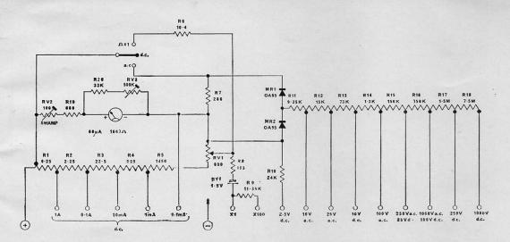
CIRCUIT DIAGRAM THE MULTIMINOR Mk. 4
