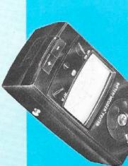
A pocket-sized instrument for testing domestic and industrial wiring and appliances.
