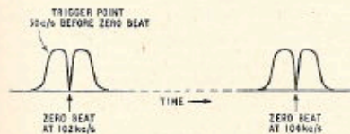
Fig. 2. Output amplitude/time characteristic of amplifier (9) during operation.
