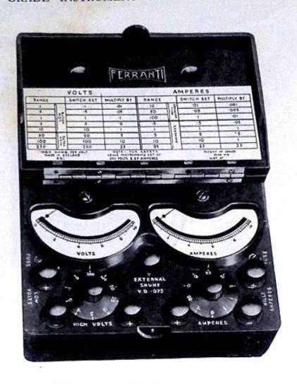
Two models are available, the essential difference being that one reads up to 250 volts, whilst the other reads up to 600 volts. The resistance of the 250 volt Instrument is 1,000 ohms per volt, whilst in the case of the 600 volt Instrument, it is 500 ohms per volt.
