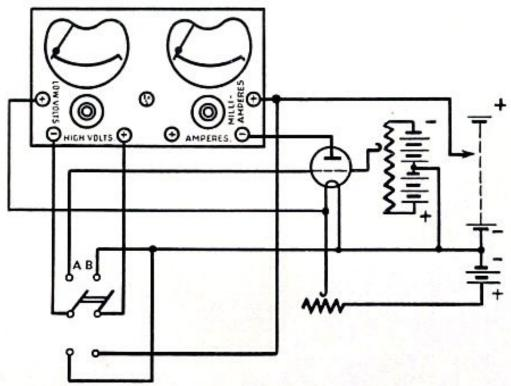
This figure shows the connection of the Test Set for taking a complete set of valve characteristics. It is most convenient to insert the valve under test in a separate holder mounted on a testing board fitted with regulating resistances and potentiometers to control the Filament Voltage, Anode Voltage and Current and Grid Voltage. An external double-pole double-throw switch has to be provided for use with the voltmeter to enable it to read the Anode, Grid and Filament Voltages.
