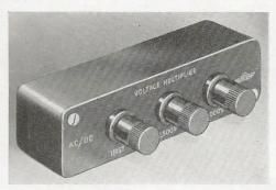
For 2,500 and 5,000 volts. The resistances are housed in a moulded box fitted with three suitably insulated terminals. When connecting in series with the Test Set, the main selector control of the latter should be turned to the 1,000 volt range, and the common terminal on top of the box should be connected to the Test Set by one of the leads supplied with it. Heavily insulated leads are supplied with the Voltage Multiplier.
